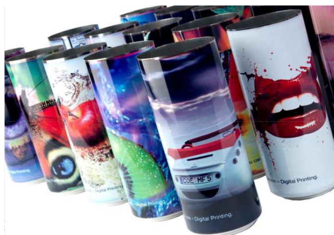
Figure 2: Photo of Metal Cans Printed with Tonejet Technology, Prior to Crimping and Capping
