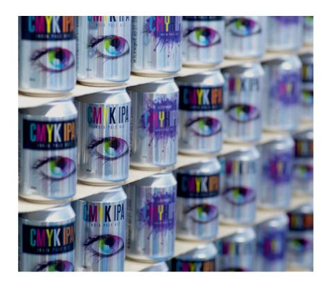
to enable them to retain their independence and uniqueness, while producing high quality bespoke products – beers brewed with varying ingredients, in relatively small batches and created for special events. One such technology is direct to can digital printing.
